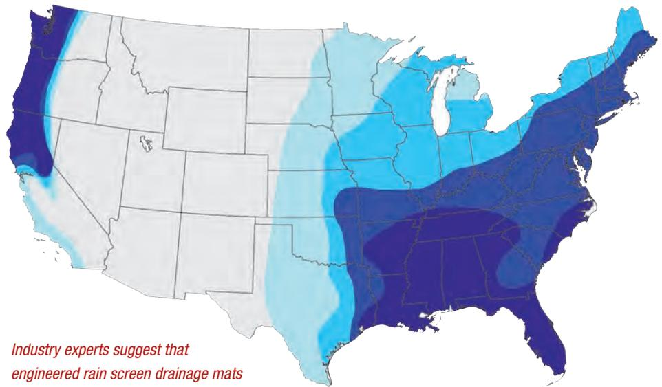
*Industry experts suggest that engineered rain screen drainage mats should be used geographically where there is twenty-inches or more of rainfall annually. Blue areas on the map should be using engineered drainage and ventilation mats.*
