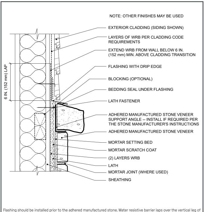
flashing should be installed prior to the adhered manufactured stone. Water resistive barrier laps over the vertical leg of flashing for positive drainage. Optional support angle shown. Verify installation requirements with adhered manufactured stone veneer manufacturer.
