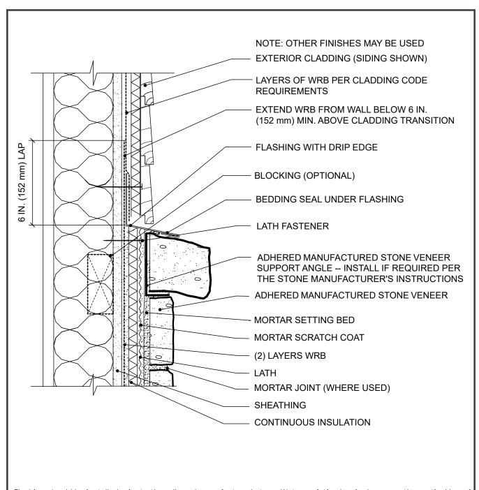
Flashing should be installed prior to the adhered manufactured stone. Water resistive barrier laps over the vertical leg of flashing for positive drainage. Optional support angle shown. Verify installation requirements with adhered manufactured stone veneer manufacturer.
