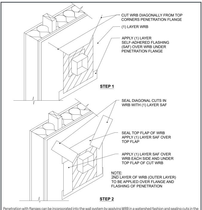
Penetration with flanges can be incorporated into the wall system by applying WRB in a watershed fashion and sealing cuts in the WRB with self-adhered flashing. Drawing illustrates installation with housewrap WRB. Installation with building paper WRB would be similar but instead of 45 degree cuts, fit last piece of WRB on top of flanges and tuck under WRB course above penetration.
